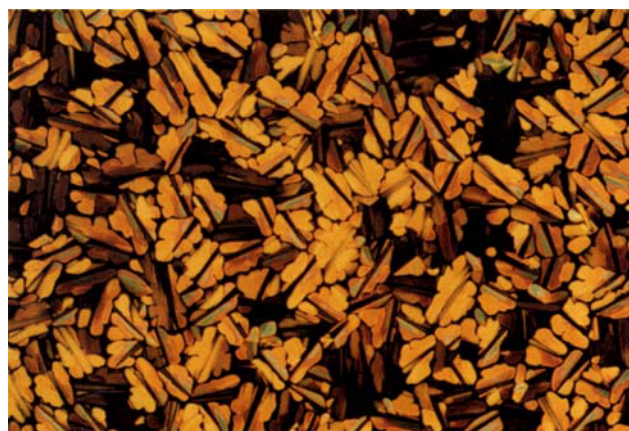
Figure 5. The dendritic texture of the mesophase of the iodo-bridged tetrapalladium liquid crystal 1c ( R = \text{C}_{12}\text{H}_{25} ) at 220^{\circ}\text{C} on cooling, magnification \times 100 .
